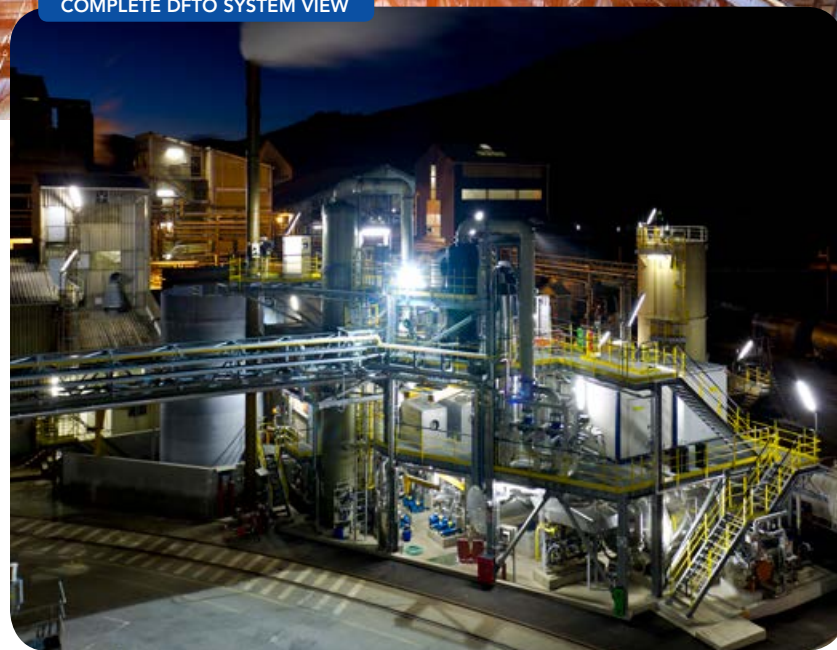
Figure 5. This DFTO system helped reduce fossil fuel use in boilers and eliminated offsite waste disposal costs.
