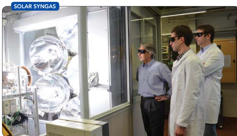
Figure 3. Process uses concentrated sunlight to convert carbon dioxide and water into a syngas that then is used to make kerosene. Source: ETH Zurich.
