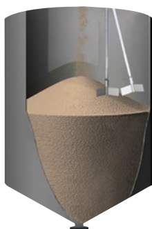
Figure 7. As material level rises in a bin, the tilt switch tips and activates a microswitch, which causes an alarm to sound.
