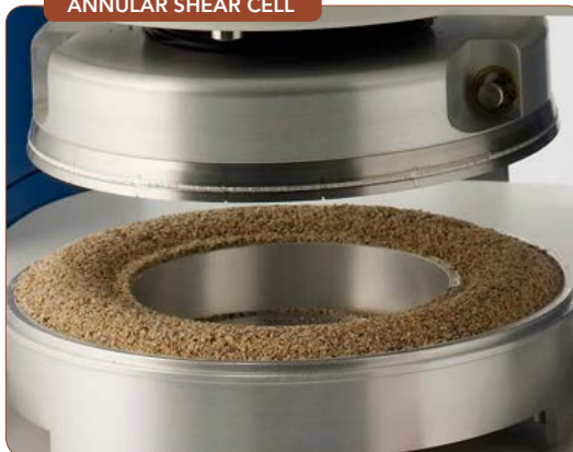
Figure 2. Shear cells can help make predictive assessments because they simulate the forces that affect powder flow in a silo.
