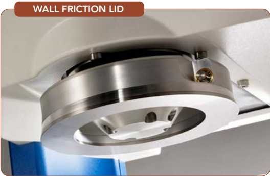
Figure 4. This lid in an annular shear cell has a smooth surface similar to the material of construction in the hopper wall.
