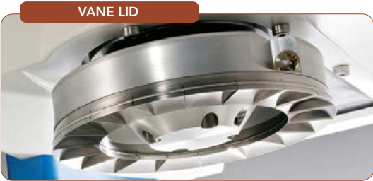
Figure 3. This shear cell’s lid has pockets separated by vanes used to measure flow.
