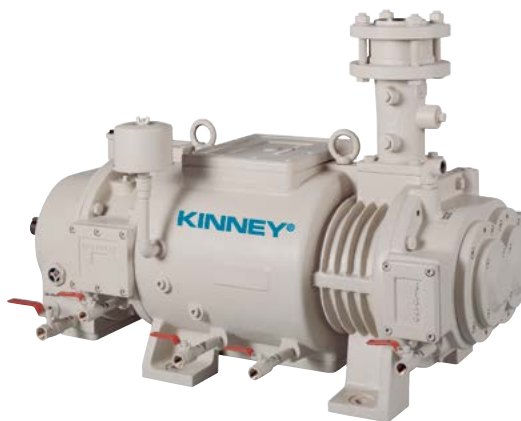
Figure 5. The rotary screw dry pump doesn't require internal lubrication and can handle some liquid carryover, it's preferred to keep the pump dry for optimum performance.
