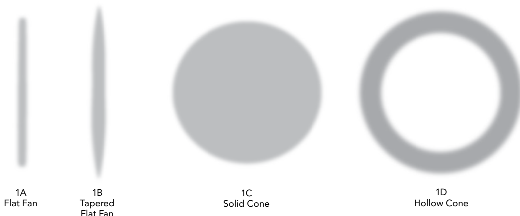
Figure 1. Nozzles use internal elements and flow passages to create the desired pattern.
