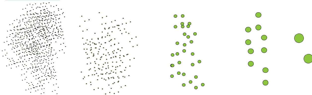
Figure 4. Nozzles can produce sprays that have different populations of droplet sizes.
