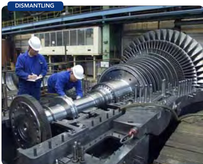
Figure 1. Steam turbine is being prepared for repair and renovation. Source: Siemens.
