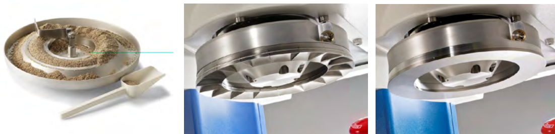
Figure 1. The basic components for an annular design shear cell include the trough with powder sample and filling accessory (a), vane lid (b), and wall friction lid (c).
