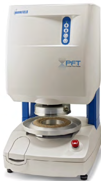
Figure 2. A typical shear cell can fit easily onto the work bench in a QC or R&D lab and can process a single sample in as little as 12 minutes.
