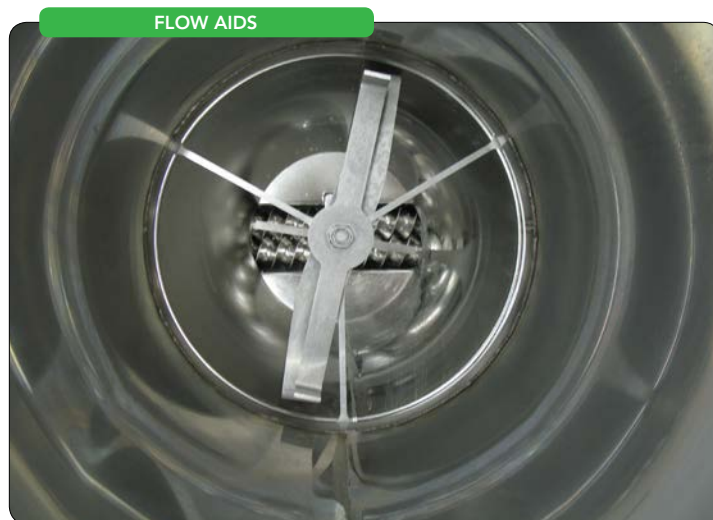
Figure 1. Cohesive materials like to pack like a snowball and need flow aids such as internal agitation, air sweeps, or air pads to create movement or external vibration to break up the clumps.
