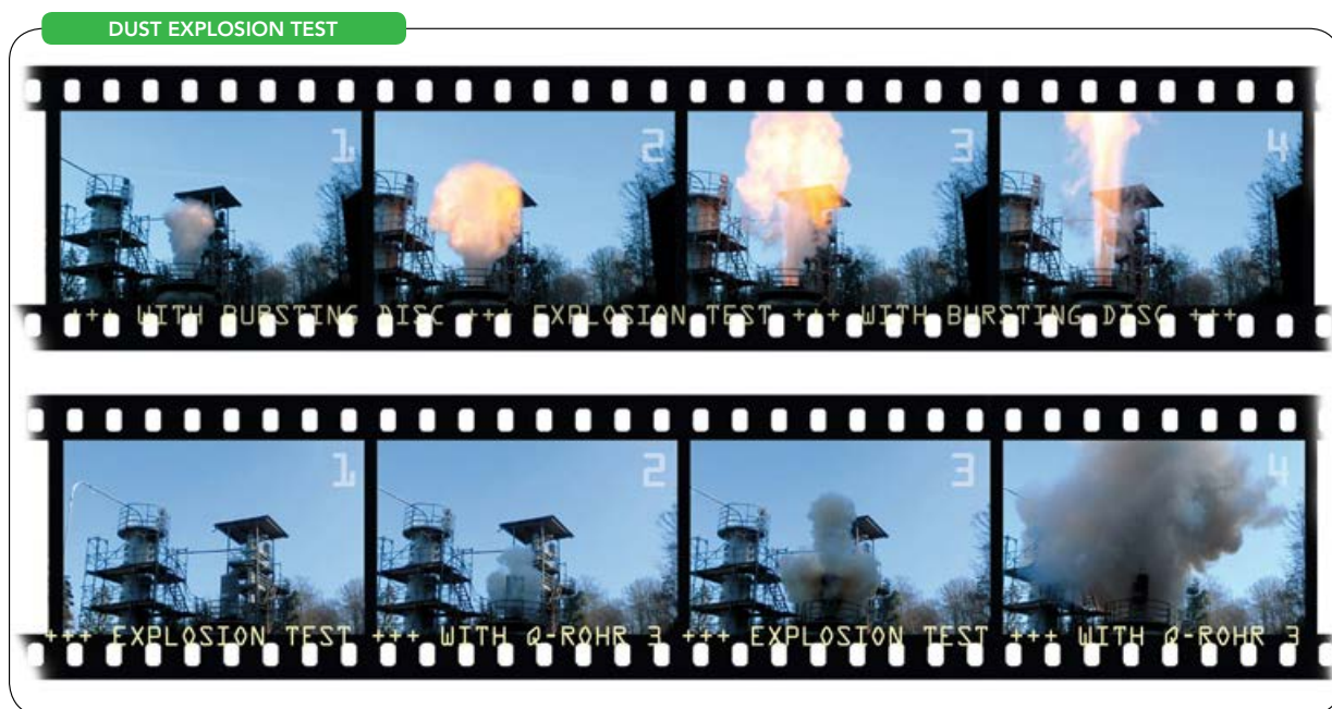
Figure 5. The first explosion test (top) uses explosion panels and produces a visible flame. The same test is performed again using the Q-Rohr-3 flameless venting system (bottom).
