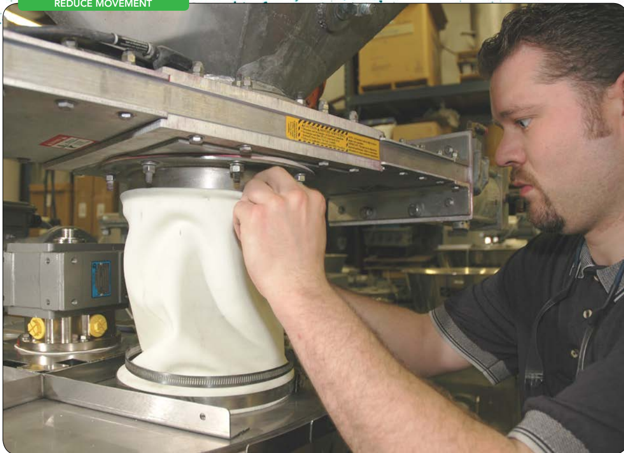
Figure 2. Any electrical, plumbing, or other connections to the gravimetric feeder must be made with flexible conduit, piping or tubing to have minimal effect on the movement of the gravimetric scale.
