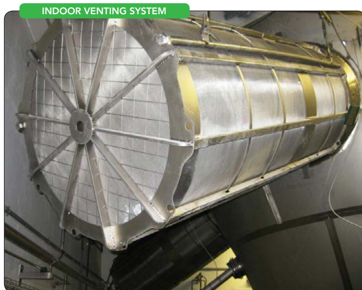
Figure 4. Explosion flame temperatures that reach up to 1,500°C (2,732°F) are efficiently cooled down through an energy transfer taking place in the unique stainless steel mesh filter basket.
