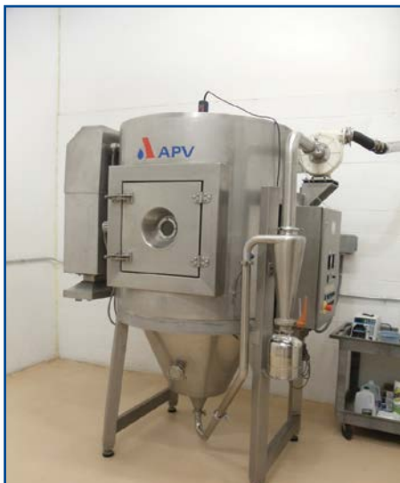
39" APV Pilot Spray Dryer, S/S
