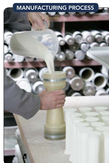
Figure 2. Oxide ceramic powder is poured into a mold.
