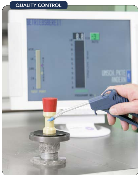
Figure 7. A helium leak test is performed to ensure quality control of the finished measuring tube.
