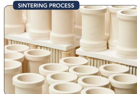
Figure 5. The ceramic is sintered in the kiln.
