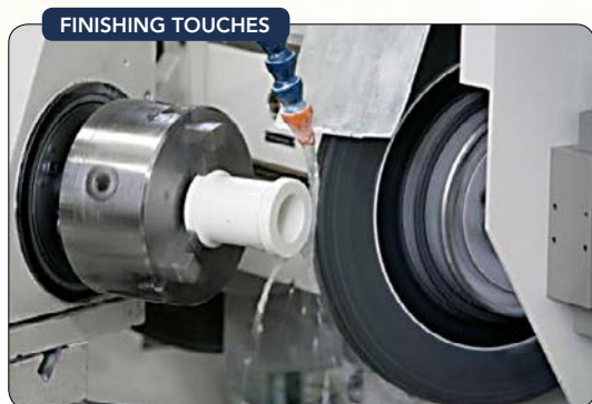
Figure 6. A diamond-tipped tool is used to machine the outside diameter, end faces and inlet taper to complete the final finishing touches of the hardened measuring tube.
