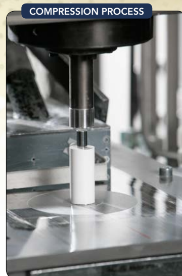
Figure 3. The powder is placed under high pressure and compressed into a cylinder.
