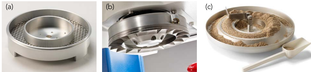
Figure 1: Components of an annual shear cell include the powder trough (a) vane lid (b) configured for uniform shearing action. A filling accessory (c) can help to fill the trough with the powder sample.
