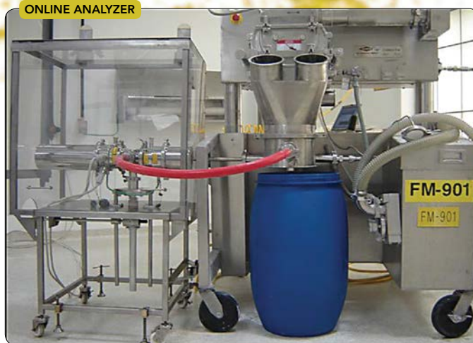
Figure 3. Device is fully integrated with mill, enabling automated control which has boosted quality and throughput and cut waste. Source: Malvern Instruments.
