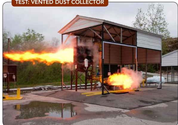
Figure 2. In this demonstration test at Fike Corporation, a flame propagates through a vented dust collector equipped with two pipes. Source: Fike Corporation
