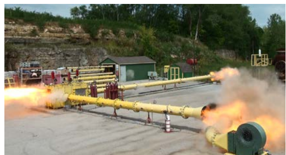
Figure 5. This series of pictures illustrates how an explosion propagation from a conveyed vented vessel is possible both with and against process flow. Source: Fike Corporation.
