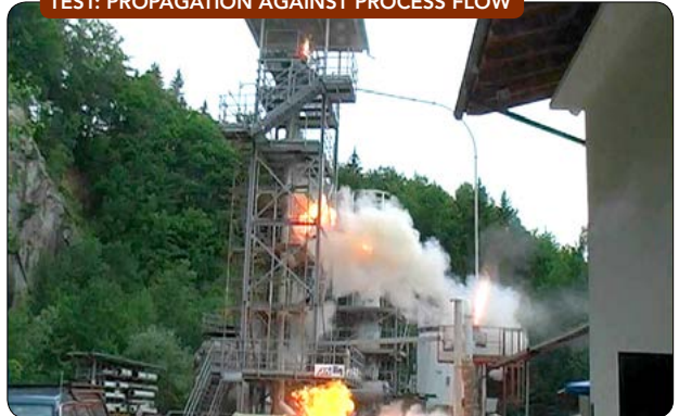
Figure 4. Dust explosion propagation tests demonstrate that an explosion is capable of traveling both with and against process flow. Source: FSA Germany.
