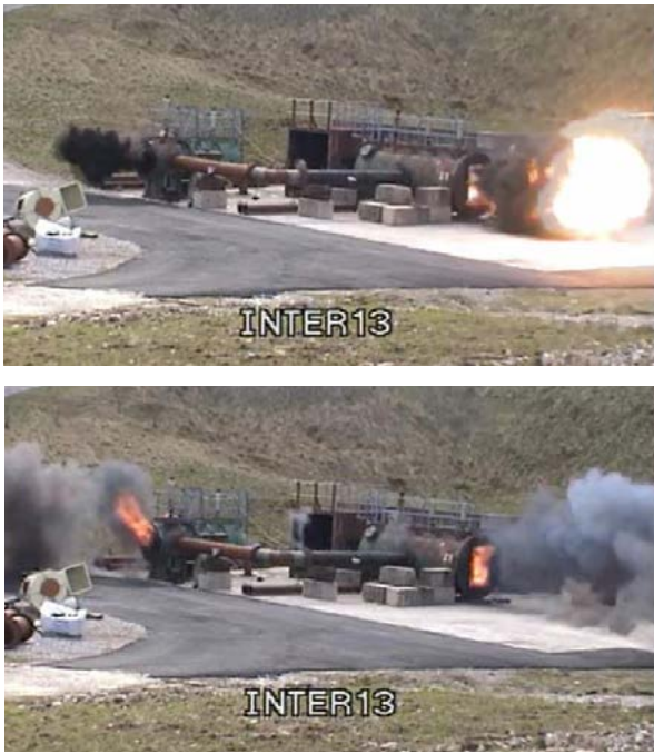
Figure 1. Explosion test is conducted using interconnected vented vessels. Source: Health and Safety Laboratory, Harper Hill, Buxton, U.K.
