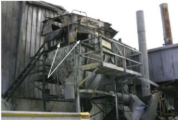
Figure 4. Dust explosion propagation tests demonstrate that an explosion is capable of traveling both with and against process flow. Source: FSA Germany.
