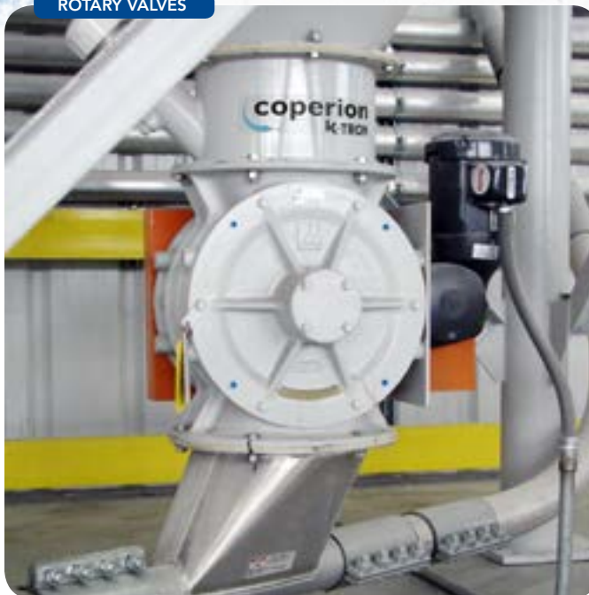
Figure 1. When selecting a dispensing device, rotary valves, such as the one shown here, are particularly useful for light, fluidizable solids that may flood the conveying lines.
