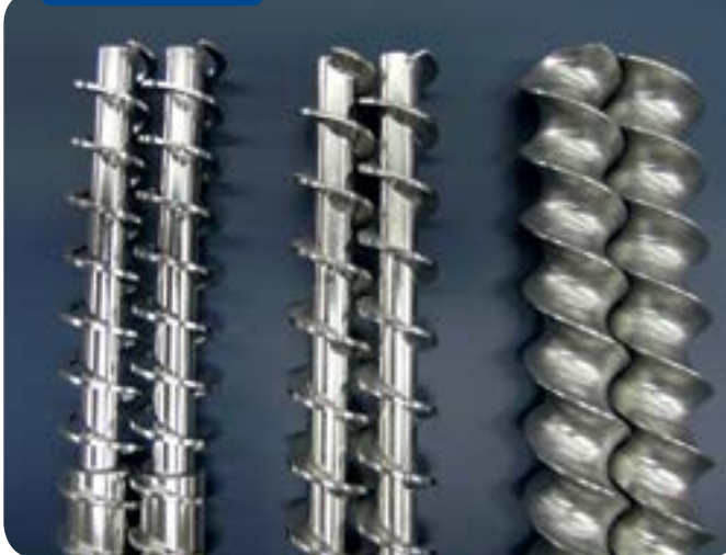
Figure 5. These intermeshing twin screws can prevent flooding of fluidized material. A variety of feeder screw designs are available, depending on the flow rate and characteristics of the mineral filler.
