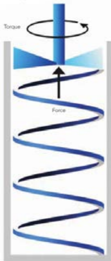
Figure 2. Powder can be subjected to different stress regimes by rotating the blade upward or downward, and air can be introduced for measuring aerated energy.
