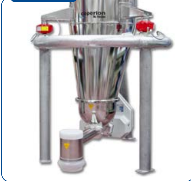
Figure 4. To prevent flooding with free-flowing grades of \text{CaCO}_3 , twin-screw feeders are recommended.
