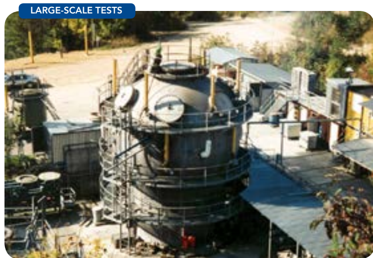
Figure 9. A 250-m 3 explosion test chamber fitted with Fike 50 L suppressors (white colored containers) is used for large-scale testing.
