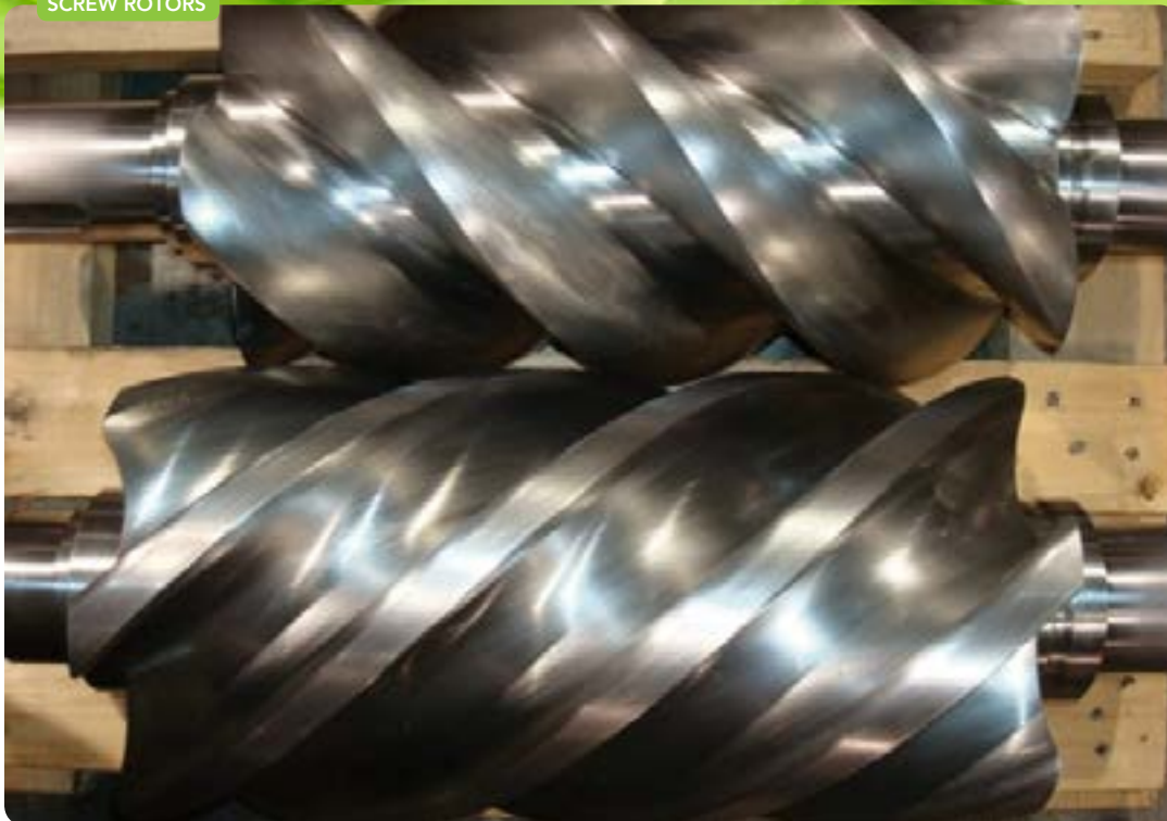
Figure 1. A higher length-to-diameter ratio increases capacity at a given speed but may decrease permissible differential pressure.
