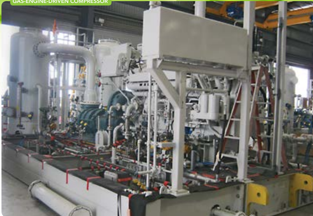
Figure 3. Large screw compressor is mounted on package skid (heavy-duty baseplate) near the suction drum and the oil separator vessel (vertical vessels).
