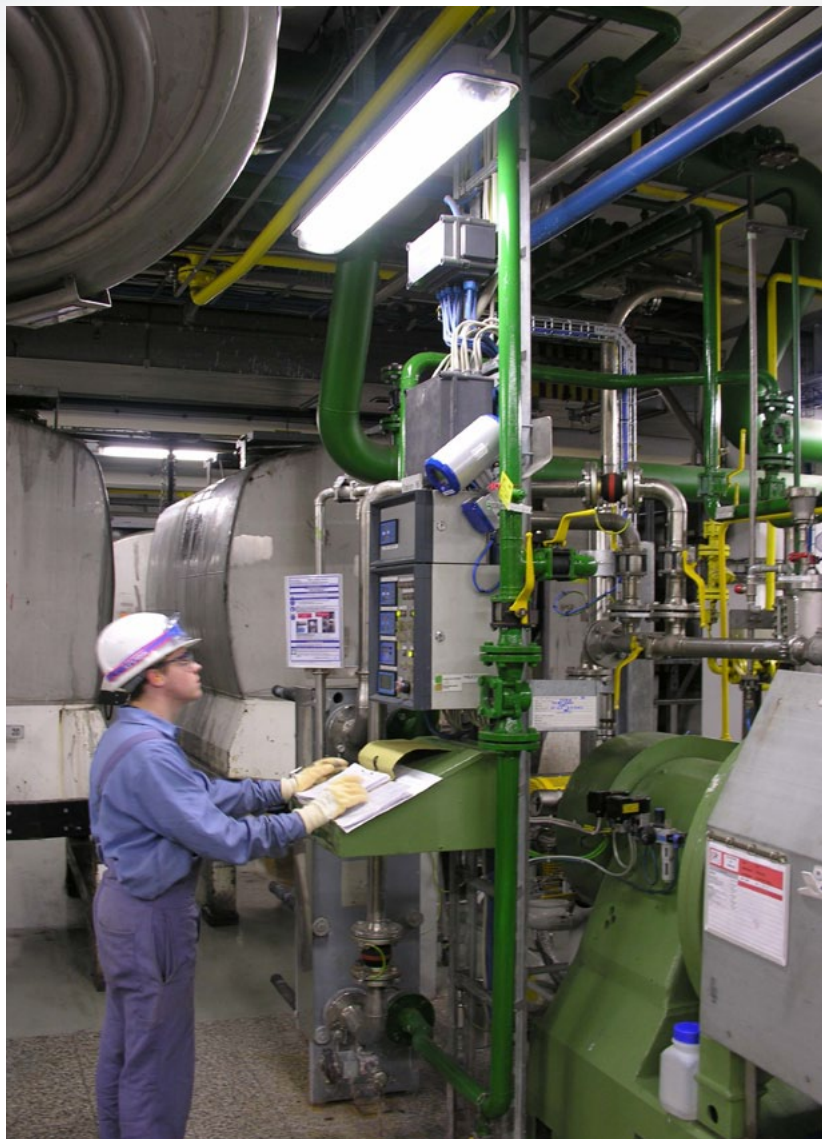
Figure 2. The varnish grinding system at BASF Coatings is designed for a flow rate of approximately 5,000kg/h.
