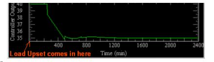
action. Because of the dead time, this is the fastest possible response for ANY feedback controller. Another dead time passes until the process settles.
