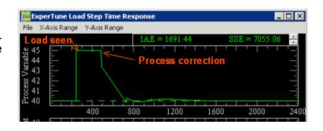
The load comes in at time zero, but because of the dead time, the process variable doesn't see the upset until 240 minutes or 4 hours later. At this time, the controller responds, but another 240 minutes of dead time go by until the process variable responds to this controller
