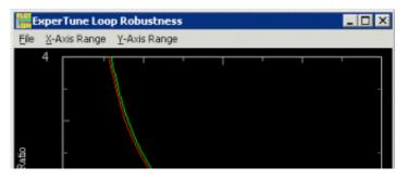
the dead time of the process can go up or **down** and the loop will go unstable. Increasing dead time with any process will always eventually drive you unstable. But decreasing dead time to make you unstable is weirdly counter-intuitive. If the dead time were to go down with a PI controller, the loop would remain stable. Let's try this in our test process to see.
