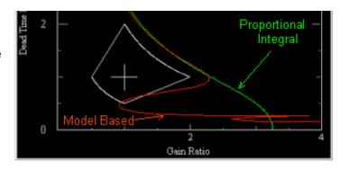
Here are the responses when we reduce the process dead time to 2 hours. The PI controller gets slower as expected. Consistent with the robustness plot, the Model Based controller goes unstable.
