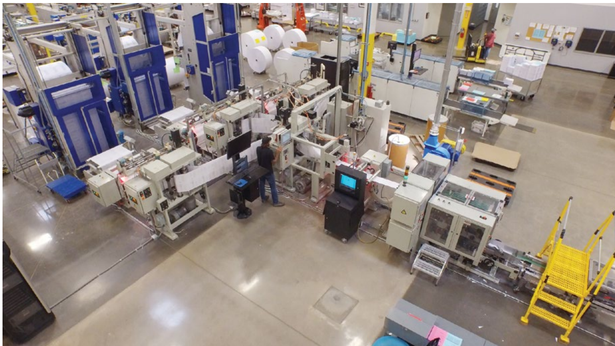
Figure 2: Once the fold is complete, the web travels through a shear-slitting module where the folded web can be trimmed, and then into the variable data rotary cutter that cuts each page to size and collates/stacks the finished product for the next process, such as final binding or saddle stitching.
