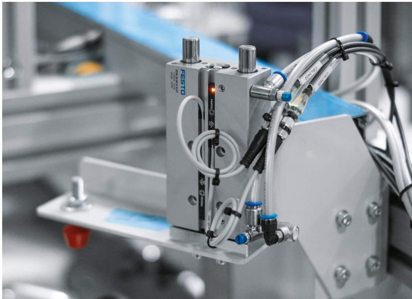
The DFM base model series is Festo's most popular pneumatic guided drive.
