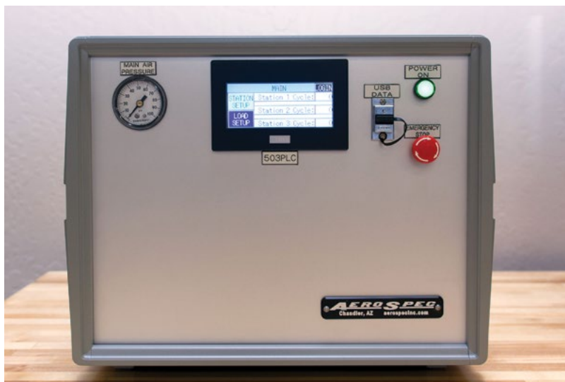
Figure 3: The HMI screen is configured to show all of the test parameters of interest and to guide the operator through the test procedures.
