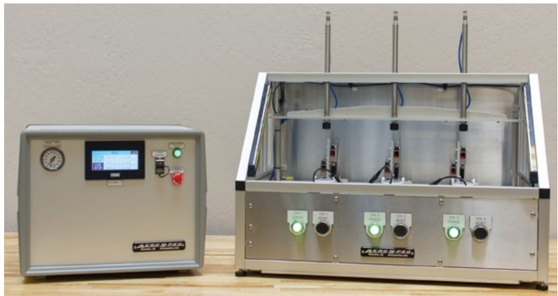
Figure 1: The heart of this medical device test system is the PLC+HMI, which performs control and monitoring of the system and provides operator interface.
