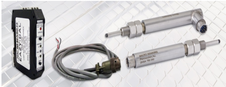
Photo 1: AC-operated LVDT gaging probes interface with single channel LVDT signal conditioners that provide either a low noise 0-10V DC or 4-20mA output for computer readout of dimensional or position measurement.
