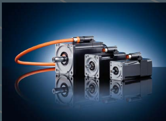
Figure 5: One recent advance designed to simplify and streamline the deployment of drive solutions is the combination of voltage supply and digital encoder signal in a single cable between the motor and drive. Half the wiring also means less mass, which can improve the efficiency of movable axis applications.
