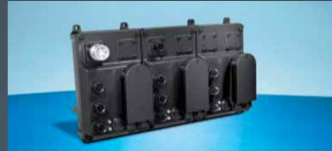
Figure 6: Three-in-one Distributed servo drives come in a variety of form factors. This machine-mountable unit includes power supply and controllers for three separate servo motors as well as local I/O and network connections.
