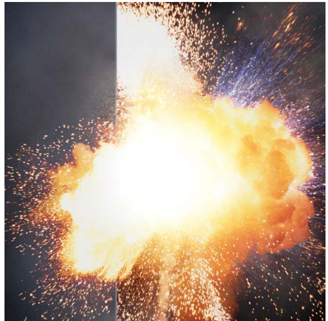
Figure 1: Arc flash explosions can be as hot as 35,000 °F, and can send shrapnel and molten metal flying out from equipment.
