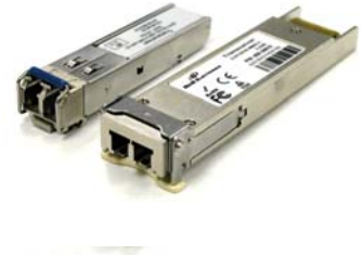
Figure 4. SFP and SFP+
