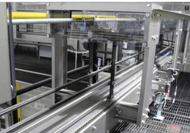
Dual lane automatic guide rail system utilizing electric actuated cylinders.
