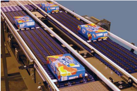
The Live Roller Metering / Merging conveyor system shown here is handling overwrapped products.
