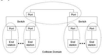
(b) Switch-based CSMA/CD network
