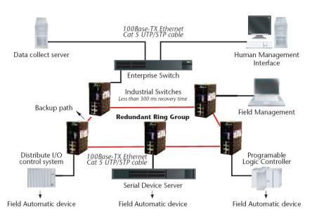
For link failure, the redundant ring group is self-healing, and recovery proceeds without human intervention. If a ring group switch fails, only the devices attached to that switch would be cut off from the network.
