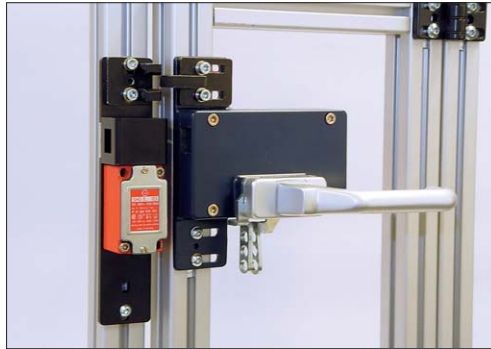
Image 3: This new door catcher ensures a proper closing of the guard door as well as a smooth insertion of the actuator in the solenoid interlock.
