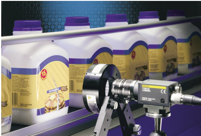
Vision sensor detects torn label
