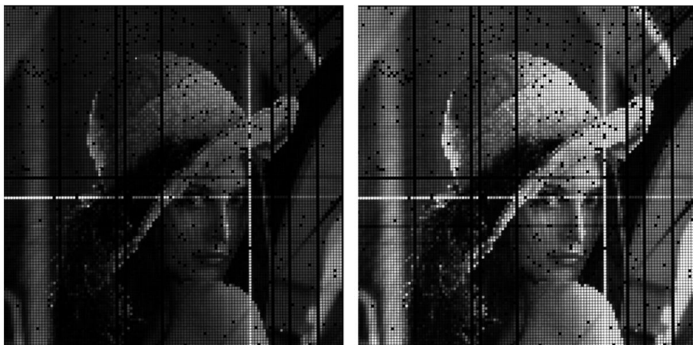
2. Test image at PWM duty cycle 100% (left), and PWM duty cycle 50% (right) (presented at the 2020 Display Week [2]).
