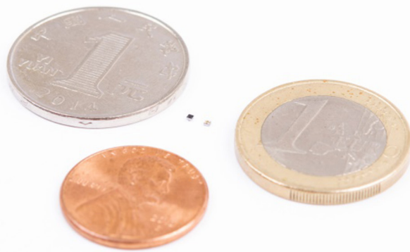
1. Coins dwarf tiny DRV5011 wafer chip-scale Hall-effect sensors, which find use in applications ranging from handheld drills to vacuum robots.
