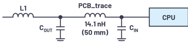
3. An LTspice model for the PCB trace inductance.
