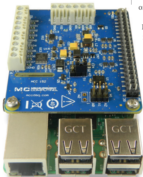
▲ Measurement Computing Corp. MCC 152 voltage-output and DIO HAT (Hardware Attached on Top) add-on board for Raspberry Pi-based systems.
