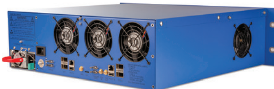
▼ Per Vices Cyan platform rear view showing QSFP+ ports
