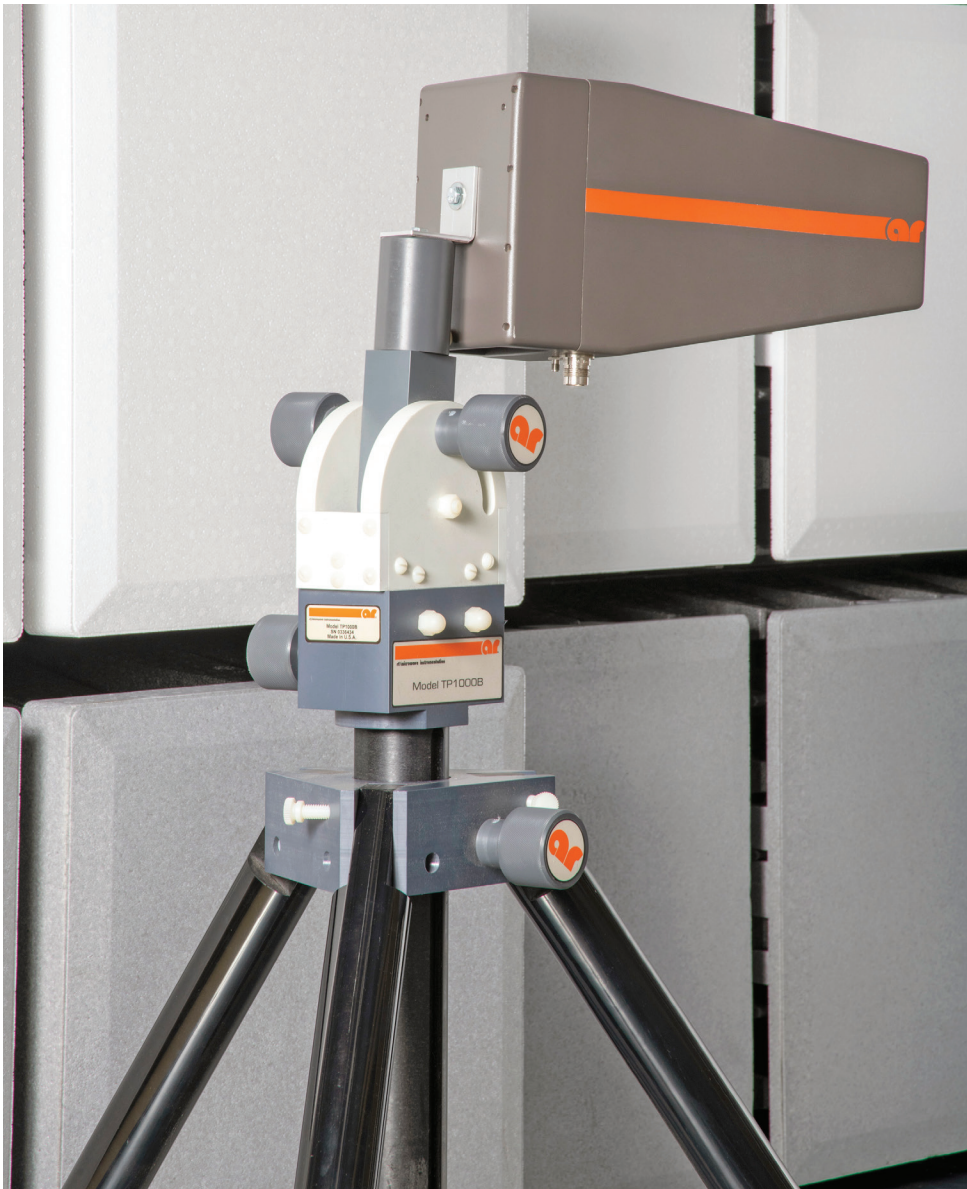
▲ AR RF/Microwave Instrumentation AA18G26-50, part of AR's AA Series of solid-state field generators.
