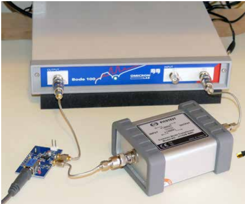
▲ Figure 3: Devices such as the OMICRON Lab Bode 100 include Picotest's Non-Invasive Stability Measurement technology
