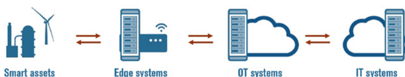
▲ Figure 1. Common Industrial IoT topology: MATLAB programs or Simulink models can be deployed on the edge, asset, or cloud.
