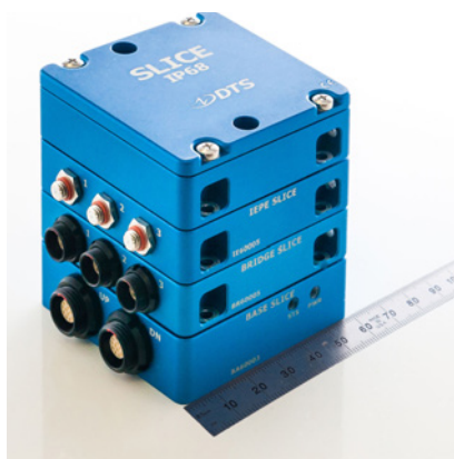
▼ Diversified Technical Systems’ SLICE IP68 is a modular, ultra-small DAQ in a waterproof, dustproof enclosure with IP68-rated connectors.
