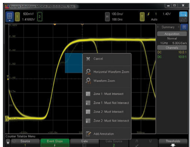
▲ Figure 2: Isolating a signal with a non-monotonic edge is as simple as drawing a box on the signal of interest and selecting “must intersect.” With normal triggering circuitry, this would be much more complicated.
