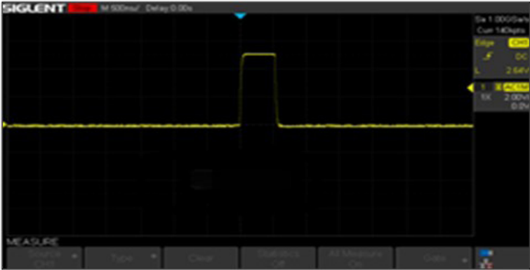
12. Oscilloscope screen capture of a typical MAX20343H HVLX waveform with 10-mA light load.
