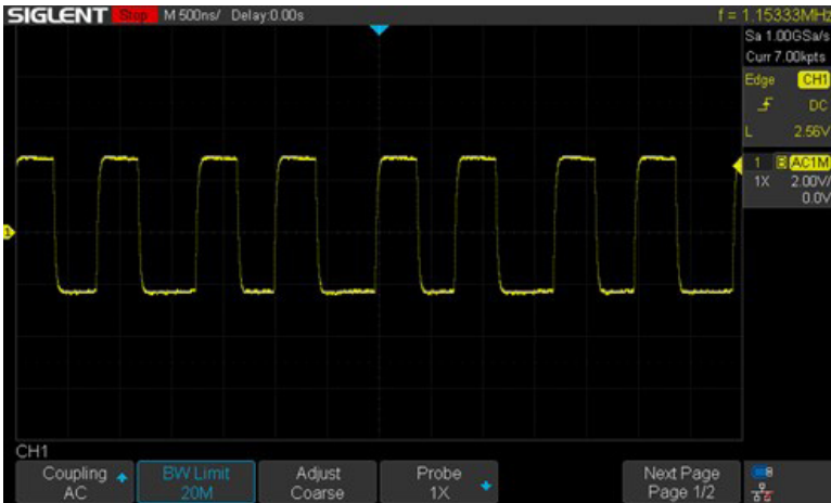
13. Oscilloscope screen capture of a typical MAX20343H HVLX waveform with 125-mA load.
