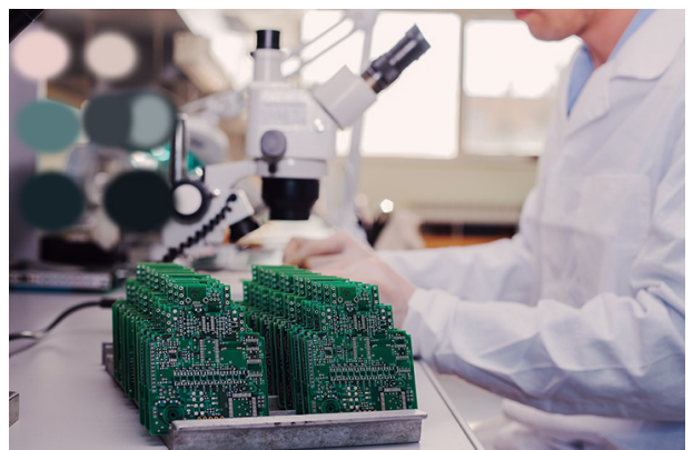
2. Manual vision inspection uses microscopes to examine printed circuit boards.
