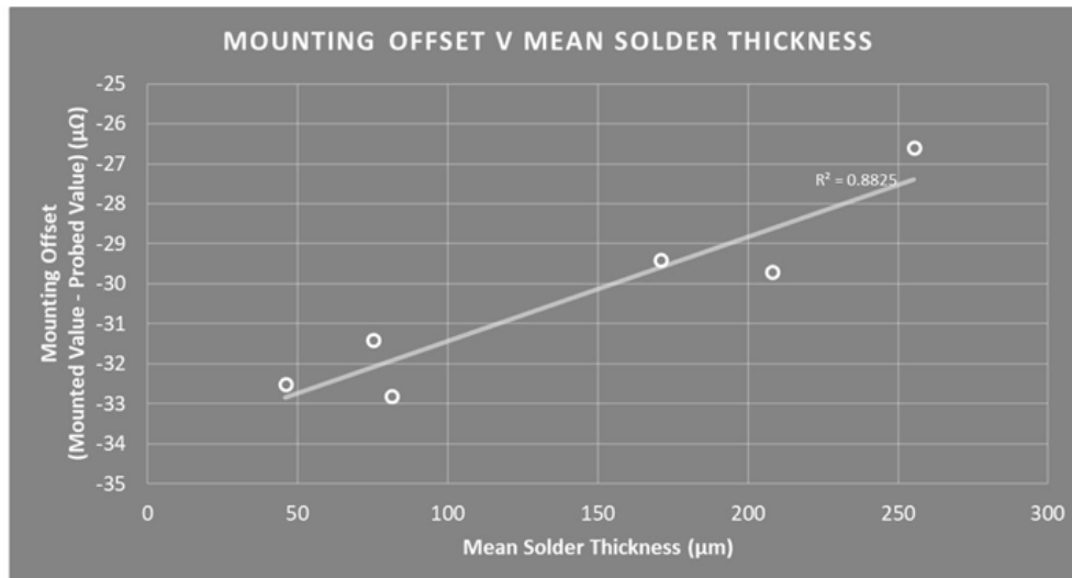
5. Shown are the results of a study examining this sensitivity in the case of the example component in Figure 4.
