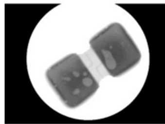
8. Voids within solder joints may have a greater effect on the mounted value if they occur in the vicinity of the voltage-sense connection (a). An X-ray of one of the mounted parts used in this study (b) gave rise to concern that the mounted value might be affected. Other samples reflowed on a different line showed very low voiding levels (c).
