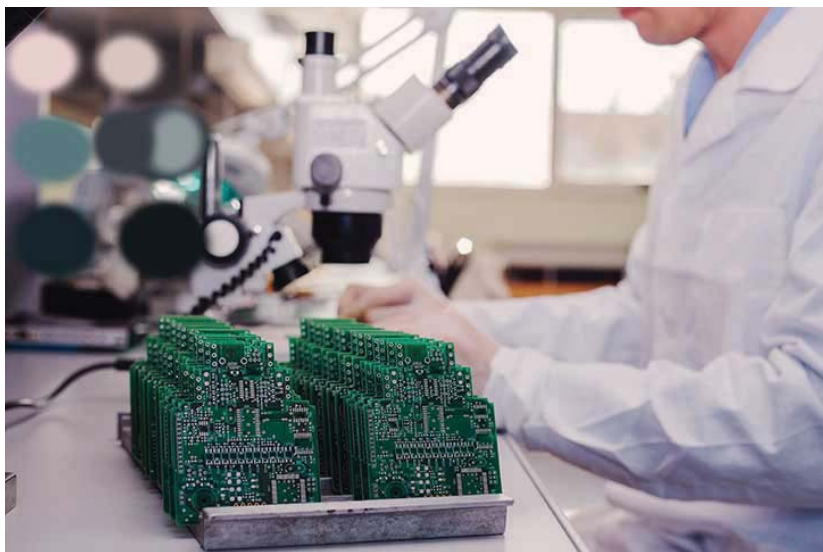
2. Manual vision inspection uses microscopes to examine printed circuit boards. Credit: Franz12, iStock
