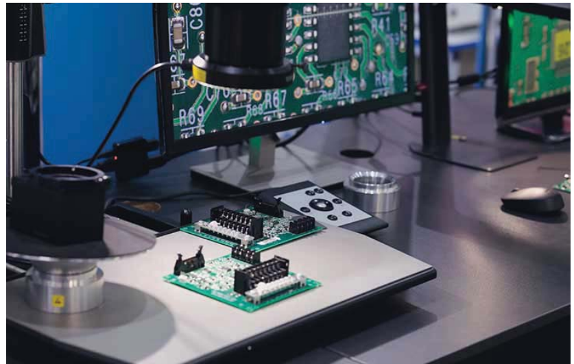
1. An inspection system with a digital microscope is used to check the quality of PCB soldering. Credit: Genkur, iStock
