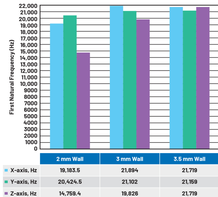
11. First significant natural frequency vs. wall thickness for the z-axis.
