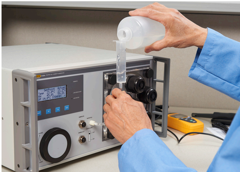
1. The Fluke Calibration 5128A RHapid-Cal Humidity Generator is a high-accuracy portable humidity generator for calibrating probes.
