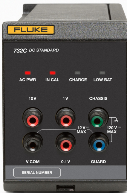
5. The Fluke Calibration 732C DC Voltage Reference Standard is based off the ampere standard.
