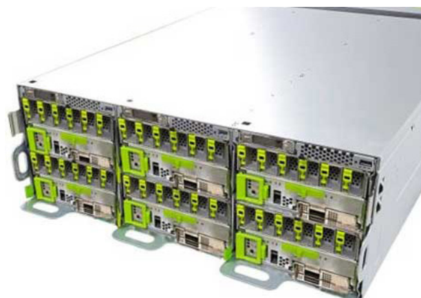
5. E1.S 25-mm SSDs are targeted for 2U and larger systems. (Source: SNIA CMSI webcast)
