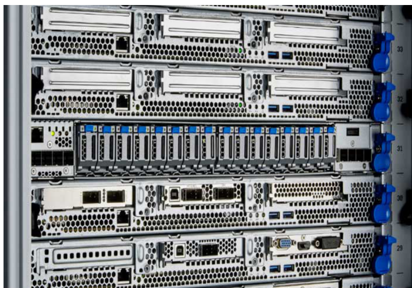
4. E1.S 15-mm SSDs are targeted for 1U/2U/4U systems. (Source: SNIA CMSI webcast)
