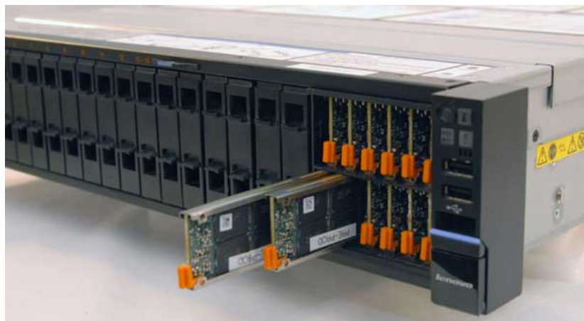
3. E1.S 9.5-mm SSDs are targeted for small footprint systems. (Source: SNIA CMSI webcast)
