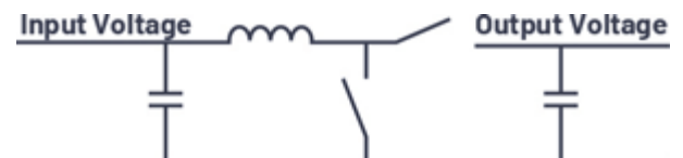
4. Concept of a simple boost step-up converter.
