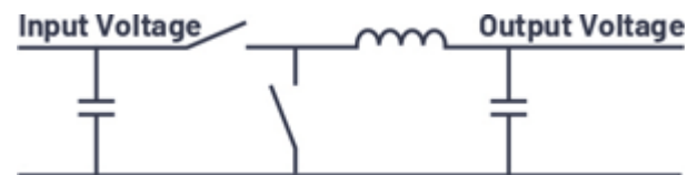
3. Concept of a simple buck step-down converter.
