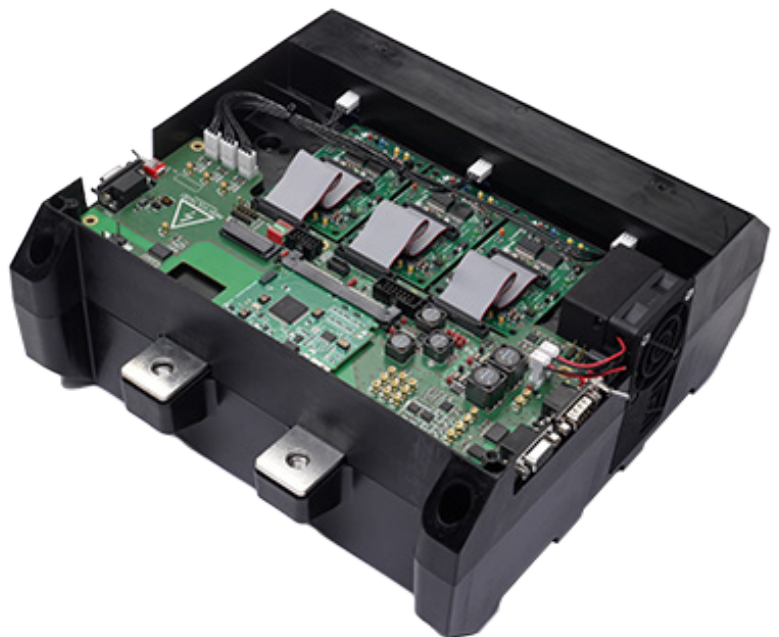
3. This fully assembled board is based on the TIDM-02014 automotive SiC traction inverter reference design.
