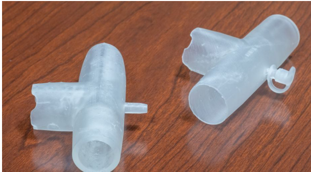
3. Northwell Health doctors turned BiPAP machines into backup ventilators by fitting them with these 3D-printed adapters. (Photo: Northwell Health)
