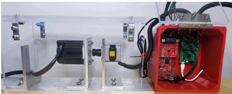
8. Here, the fully-assembled dynamometer is testing a stepper motor.
