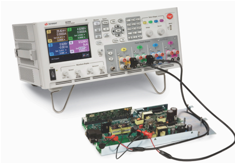
24-3. Keysight's N6705 DC Power Analyzer provides insights into the DUT's power consumption in minutes without writing a single line of code.
