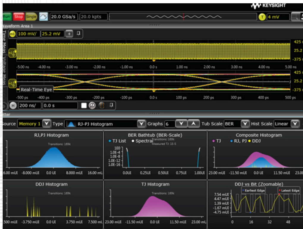
5. Jitter components are automatically separated and compared on a Keysight Infiniium oscilloscope using EZJit Complete.
