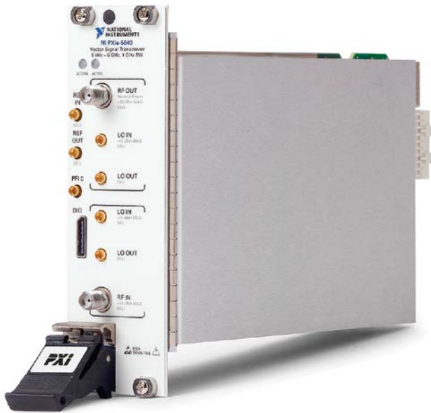
4. National Instruments' 5840 vector signal transceiver (VST) combines a 6.5-GHz RF vector signal generator, 6.5 GHz vector signal analyzer, user-programmable Virtex-7 690T FPGA, and high-speed serial interface into a single two-slot PXIe module.
