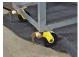
Bunched up rental rugs made it difficult to move heavy louver carts.
