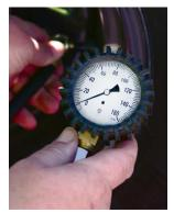
A major reason even the most well intentioned tire programs fail to achieve results is due to inaccuracy of pressure gauges as a whole. Tires are engineered with a certain pressure range in mind that creates the optimal rolling resistance for the advertised savings in fuel costs. Verifying and maintaining proper inflation is not only a matter of habit and attention to detail, but requires precision equipment.
